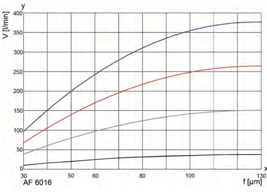
The curves represent the volumetric flow through the entire filter system (filter housing including one filter element as an example) and refer to a differential pressure of 0.3 bar. Specific information about process data is essential for reliable operation of automatic filters.
