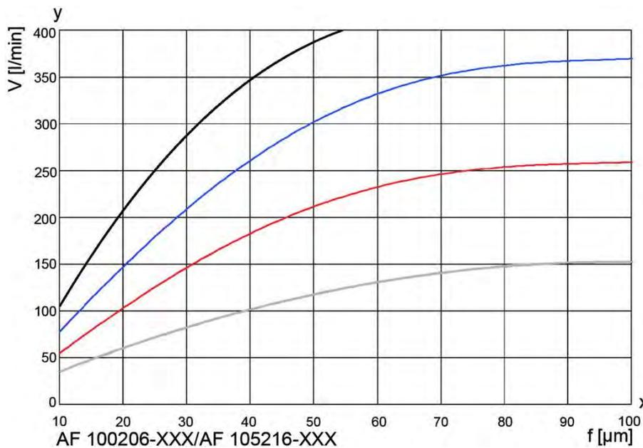
The curves indicate the volume flow through the complete filter system (filter housing including element) and are referred to a differential pressure of 0.3 bar. Specific process information is essential to guarantee reliable operation of an automatic filter.
