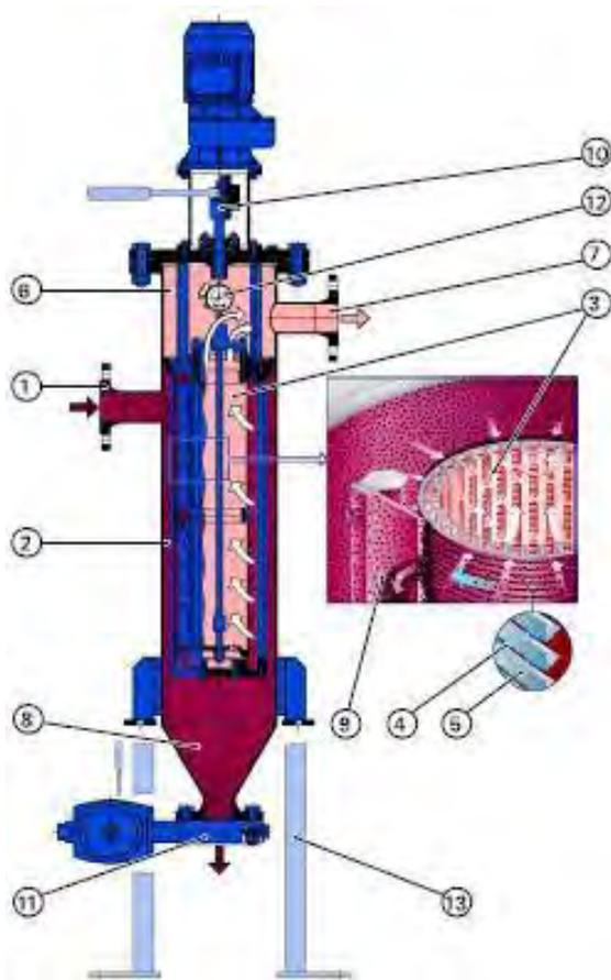
**On the FGC metal-edge filter AF 73 S, coiled cartridges, welded cartridges, and perforated foils can be used.**
