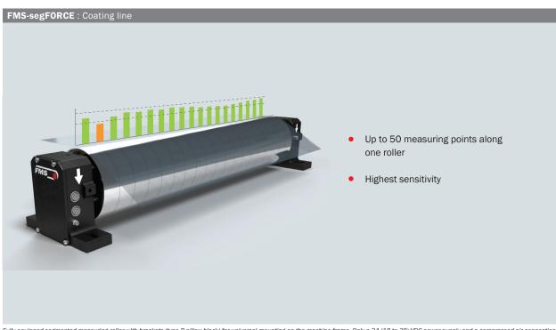
Fully equipped segmented measuring roller with brackets (type P pillow block) for universal mounting on the machine frame. Only a 24 (18 to 38) VDC power supply and a compressed air connection are required. Data connection is realized with an RJ-45 socket.
