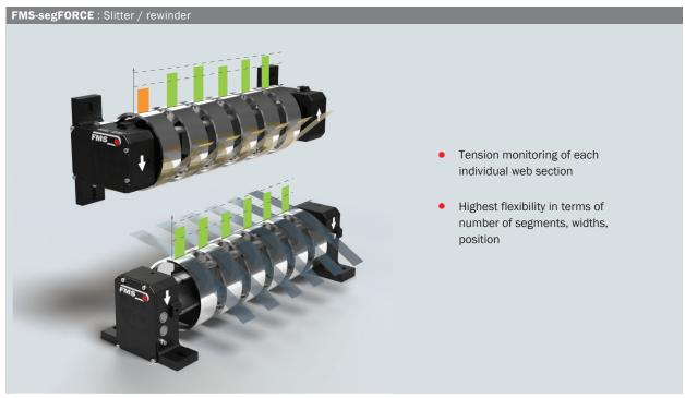
Schematic of two measuring rollers in the slitter / rewinder. The offset of the individual segments from the lower to the upper measuring roller can be seen clearly. Smallest differences in tension between the individual web sections quickly become visible. The sophisticated design allows all types of wrap angles to be covered. Flexible segment widths and freely adjustable distances between the segments make it possible to configure the measuring rollers for a wide variety of slitting widths.
