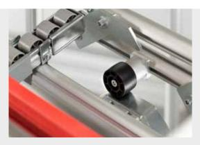
When the shooter approaches, the Roller strut moves closer to the roller conveyor as the Ramp pushes it up and to the side. This movement forces the Bars to pivot to the side. When the shooter is moved away, the pressure on the ball-bearing mounted Actuator Roller drops and the Spring-loaded Reset Device pulls the roller strut back down to the starting position.
