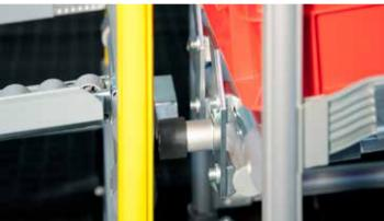
Actuator Ramps are available in two installation depths to suit different roller conveyors (38 and 61 mm). This ensures that even conveyor lines that protrude can be reliably actuated.
