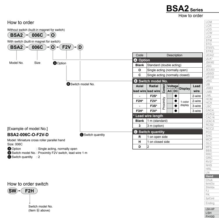
Note) When two switches are selected, the open/close stroke length will be short. Depending on workpiece size, both switches may turn ON.
