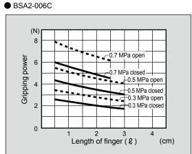
Note: O type gripping power decreases approximately 20 to 30% in the closed direction compared to double acting. C type gripping power decreases approximately 10 to 20% in the open direction compared to the double acting. When making a selection, read the precautions for design and selection on page 1764.
