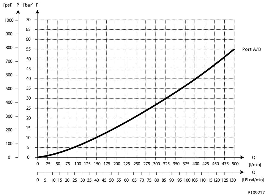
*Load Independent Oil Flow, Pressure Compensated*
