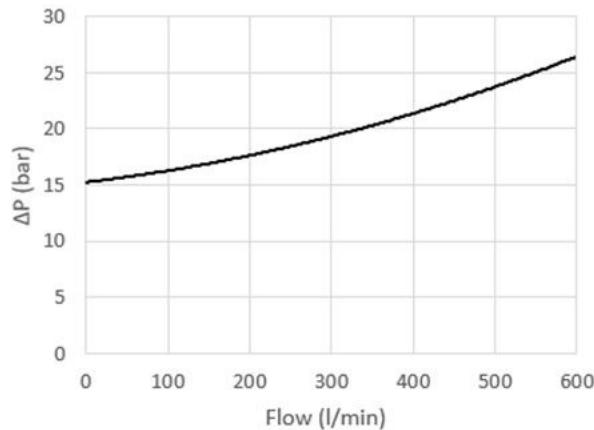
Inlet relief pressure is dependent on inlet flow rate and will follow the curves in the graphs below. The final relief setting should be made at the maximum application flow rate. This setting must not exceed the continuous pressure rating of any component in the valve stack.
