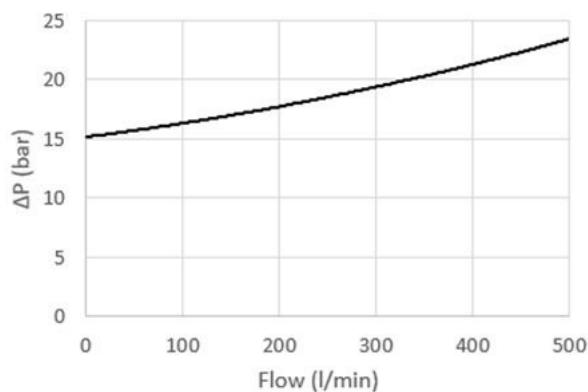
Inlet relief pressure is dependent on inlet flow rate and will follow the curves in the graphs below. The final relief setting should be made at the maximum application flow rate. This setting must not exceed the continuous pressure rating of any component in the valve stack.
