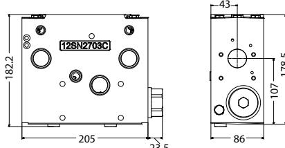
The PVG 256 Basic modules (PVB), also referred to as work sections, is the interface between the PVG 256 proportional valve group and the work function such as a cylinder or a motor.
