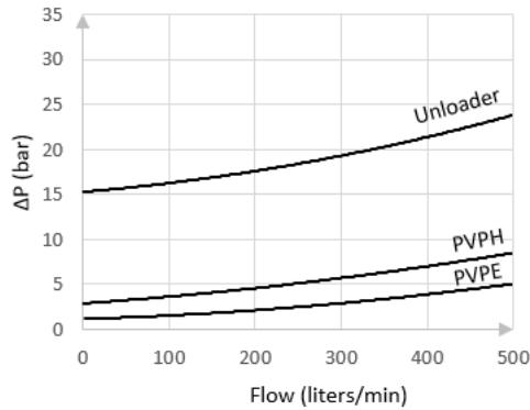
*Neutral Bypass Pressure Drop Characteristics – OC256 with PVPV256*
