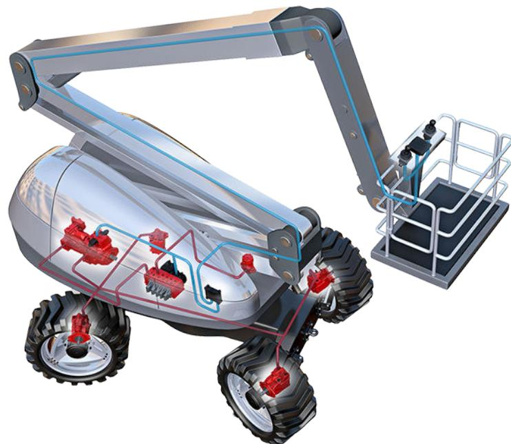
This example breaks down the control system into smaller bits explaining the architecture in depth. Even though many Danfoss components are used in the PVG control system.
