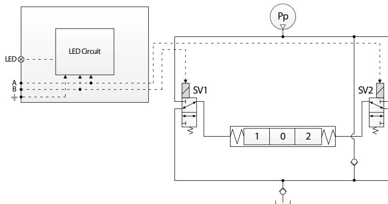
The standard PVEO functionality includes the simplest electric circuit of the PVG 128/256 actuator program, using a fixed 12 Vdc or 24 Vdc supply voltage or signal voltage and a simple LED circuit to control the LED light indicating Power ON/OFF.
