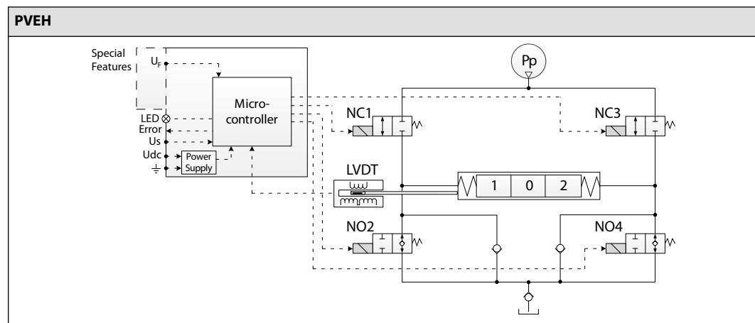
**PVE Variant Overview*****PVEH Schematics and Dimensions*****Schematics**
