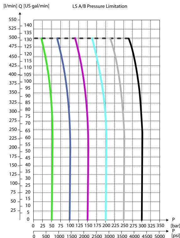
*Load Independent Oil Flow, Pressure Compensated*
