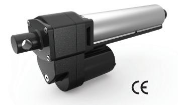
The K4x model provides the highest load rating in its class. This model incorporates all of the base K2 features with a ball screw for a 4,000 lb. (17760 N) load capability within a compact package size. The K4x includes a bi-directional wrap spring brake for load holding capability. These units are well suited for the most demanding applications where an alternative to hydraulic or air cylinders is needed or where hydraulic power sources are not available.
