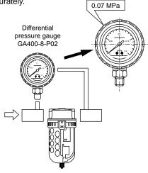
■ The micro alescer (oil removal filter) mantle (element) service life is reached when the pressure drops to 0.07 MPa. Replace the mantle with a new one at the end of its life. (Do not touch the urethane foam layer when replacing the mantle.)
