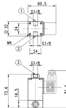
In the mod. 648-150-A6\* (NO) connections 1 and 3 are inverted.
