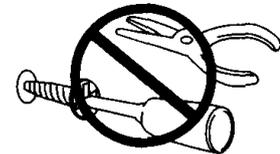
○ If the supply cord is damaged, it must be replaced by the manufacturer, its service agent or similarly qualified persons in order to avoid a hazard.
