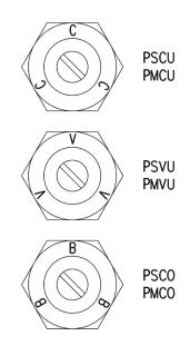
IDENTIFICATION OF DIFFERENT TYPES: PSCU - PMCU = assembly directly on the cylinders PSVU - PMVU = assembly directly on the valves PSCO - PMCO = assembly directly on the cylinders or valves
