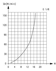
Flow Qn (Nl/min.) from  $2 \rightarrow 1$  with controller OPEN: 200 Flow Qn (Nl/min.) from  $2 \rightarrow 1$  with controller CLOSED: 70
