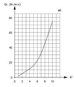
Flow Qn (Nl/min.) from  $2 \rightarrow 1$  with controller OPEN: 70 Flow Qn (Nl/min.) from  $2 \rightarrow 1$  with controller CLOSED: 33
