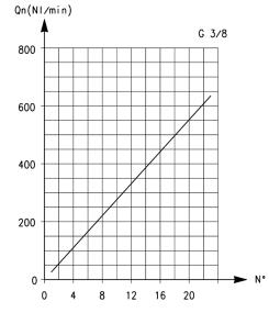
Flow Qn (Nl/min.) from 2 → 1 with controller OPEN: 710 Flow Qn (Nl/min.) from 2 → 1 with controller CLOSED: 410
