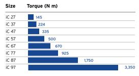
7 sizes iO 37 ... iO 97 Nominal torque ( $M_{\rm N2}$ ) up to 3,650 N m Transmission ratio ( $i_{\rm N}$ ) 5.4 ... 197
