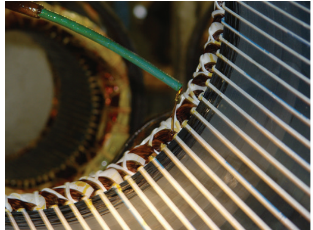
Figure 1.12.c - Resin applied by continuous flow process
