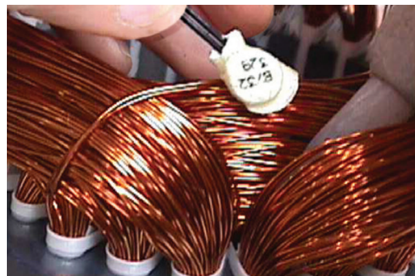
Figure 7.6 - Thermostat installation in the winding
