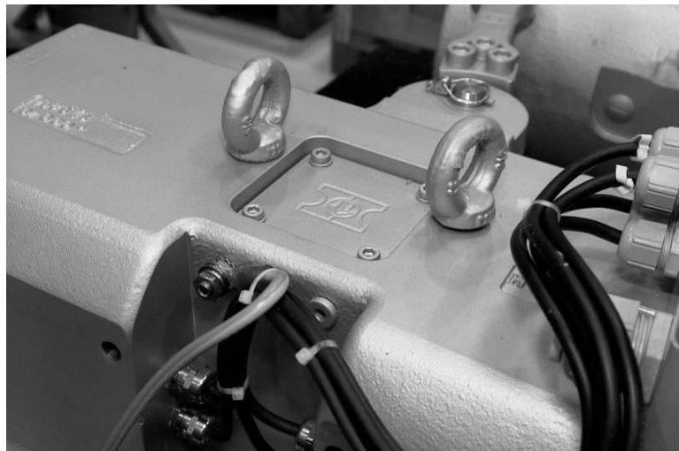
Fig. 82: Attach eye bolts to the double-acting magnet
