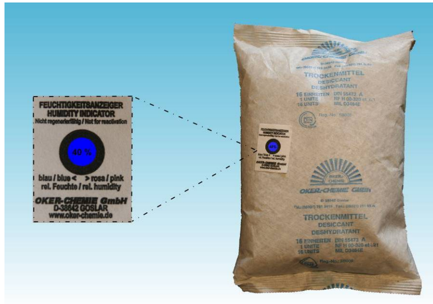
Fig. 4: Humidity indicator on the desiccant bag before use
