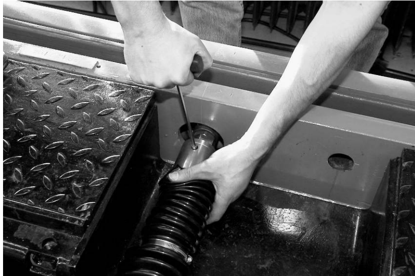
Fig. 52: Secure brass sleeve
