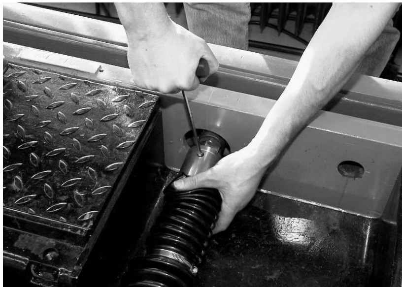
Fig. 103: Loosen the hexagon socket screw on the drive rods
