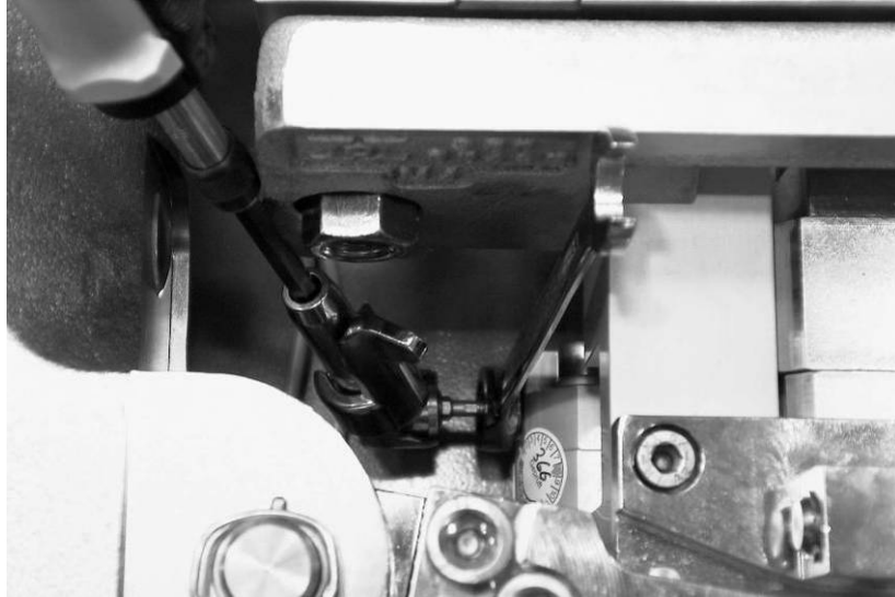
Fig. 76: Set the hydraulic damping device
