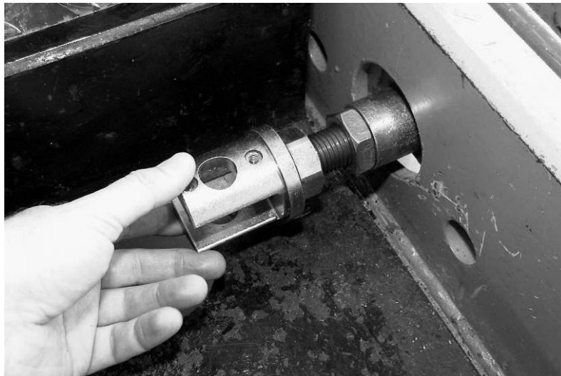
Fig. 50: Mount the connection bracket
