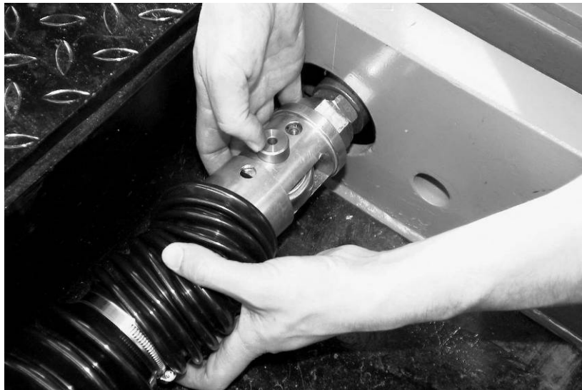
Fig. 51: Mount drive rods
