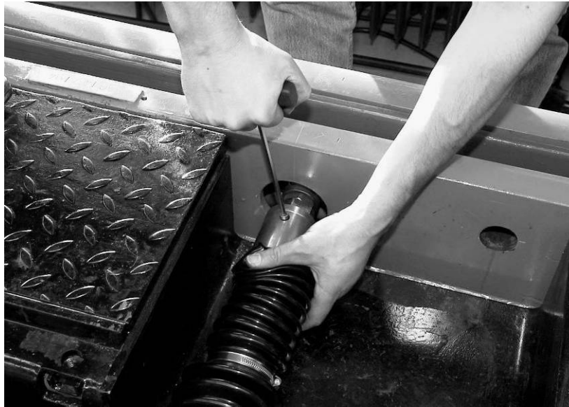
Fig. 84: Loosen the hexagon socket screw
