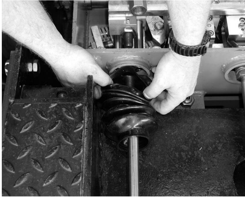
Fig. 110: Replace the bellows on the drive rods
