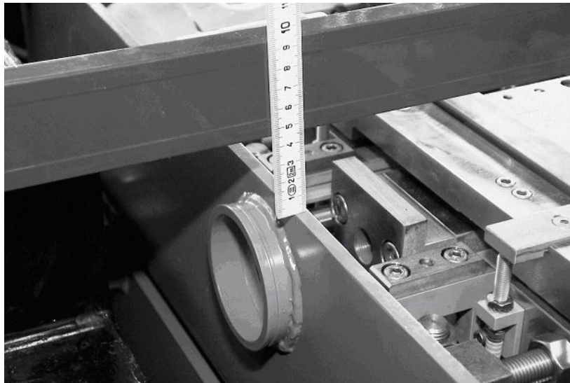
Fig. 41: Measure the clearance between the upper surface of the rail and the upper surface of the housing
