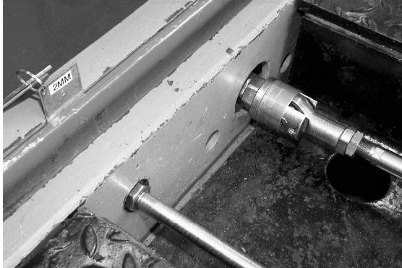
Fig. 68: Insert measuring plate 0.08 in [2 mm] - in driving direction left
