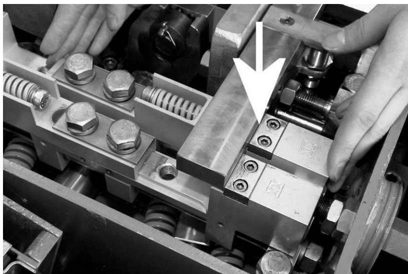
Fig. 71: Set the tongue detector lock on the open point
