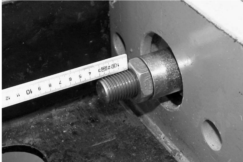
Fig. 48: Measure the remaining thread of the hammerhead screw
