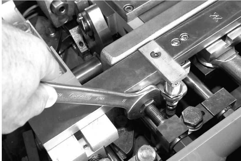
Fig. 57: Unscrew the securing nuts
