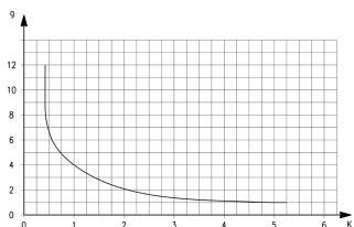
Pressurisation times as to the number of turns of the regulation screw, with downstream volume of 5 litres. A = 5 turns; B = 4 turns; C = 3 turns; D = 2 turns; E = 1 turn. K = number of turns of the regulation screw required to obtain the required pressurisation time with an inlet pressure of 6 bar. Variations of the inlet pressure can cause deviations of the pressure time by  $\pm$  20%. K = t/V where: V = volume of the downstream system in litres; t = desired pressuring time in seconds.
