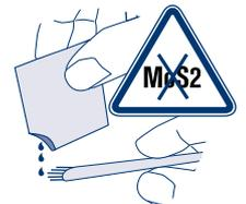
Oil hub and shaft lightly, if necessary (do not use oil containing MoS<sub>2</sub>).
