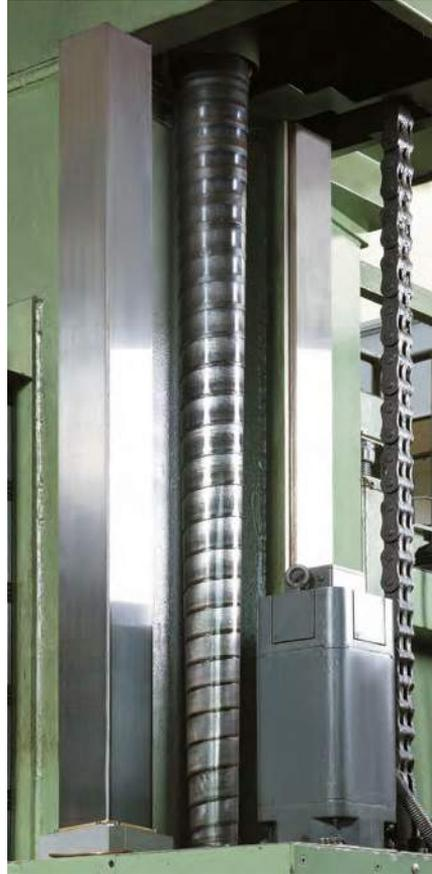
The springs are made of hardened high-quality spring band steel. The optimized design means that the horizontal bending and vertical deflection is very
