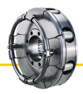
Due to unique freewheeling springs, the Black Bruin motor can freewheel without active hydraulics and work as a traditional wheel hub.
