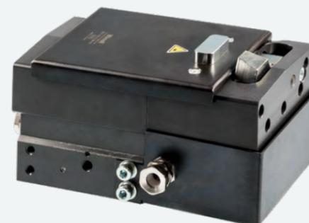
With integrated anti-bounce stop designed to keep the pallet in position after the damping operation. A sealed cover that travels simultaneously with the damping unit protects the device against dirt and aggressive liquids. The solution also includes a retracted stop sensor (damping completed but mechanism still locked) and makes it possible to lock the stop in the lower position. Ideally suited for use in harsh environments, e.g. when linking machining centers in the automotive industry.
