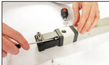
Tighten motor mounting screws
