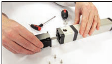
Insert motor shaft into coupling
