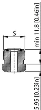
Dimensions of O-rings for 11/16-16 UN ORFS ports:  $9.25 \times 1.78$  mm [ $0.334 \times 0.0701$  in]
