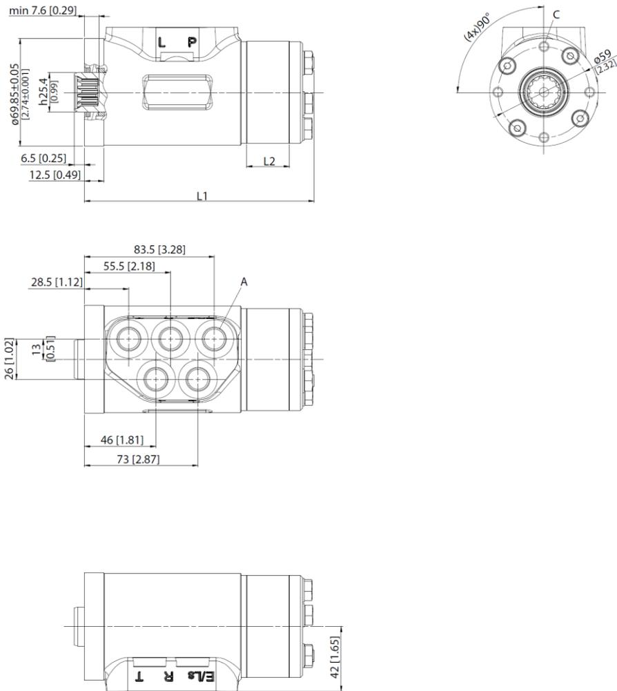
**A (P, T, L, R, and PB/LS)** 9/16"-18 UNF w/ O-ring boss and spot-face, ISO 11926-1, 12.7 mm [0.40 in] deep OR: M14 x 1.5 w/ O-ring boss and spot-face, ISO 6149-1, 11.5mm [0.45 in] deep
