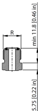
Dimensions of O-rings for 9/16-18 UNF ORFS ports:  $7.65 \times 1.78$  mm [ $3.02 \times 0.702$  in] (SAE J515 seal size no. 011). Rear-ported OSPM steering units are also available with 11/16-16UNF ORFS type.
