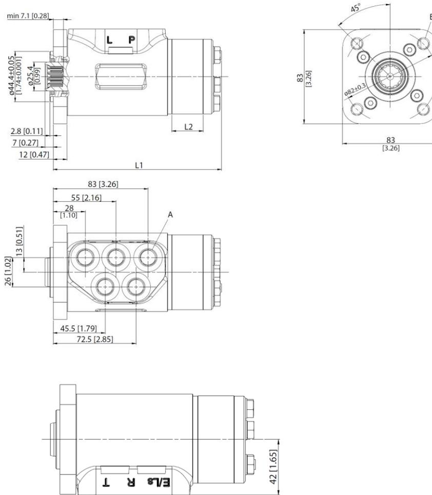
**A (P, T, L, R, and PB/LS)** 9/16"-18 UNF w/ O-ring boss and spot-face, ISO 11926-1, 12.7 mm [0.40 in] deep
