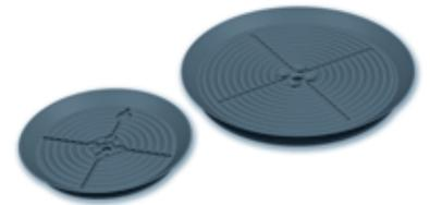
SPL suction cups are used to handle heavy loads such as sheet metal or glass panels. They have internal cleats allowing them to handle thin sheet metal without distorting them and for vertical handling (non-slip).
