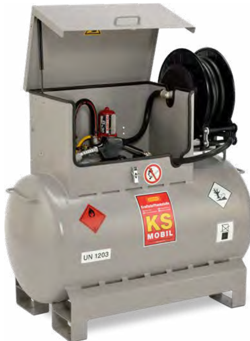
Pump cabinet (KS-Mobile 300 L) with pump 12 V, 25 L/min, ATEX, hose reel (accessory) and automatic nozzle
