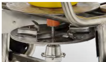
Stainless steel spreader disc, adjustable
