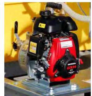
Honda pump with petrol engine 130 L/min
