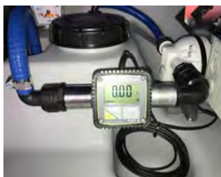
Meter FMT 3 with pulse output
