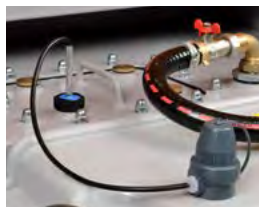
Overfill prevention sensor
