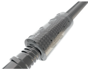
TS, Loading Non Preloaded Single Nut, B-type recirculation
