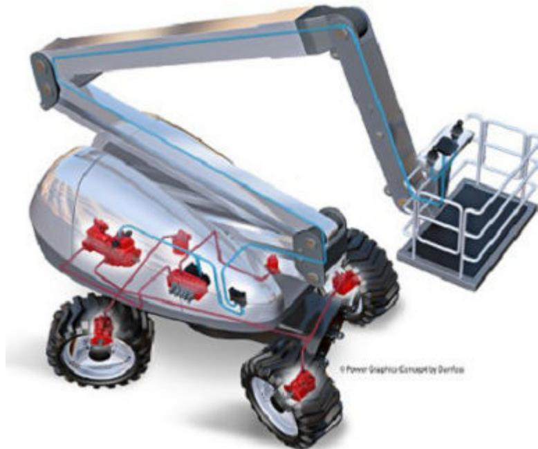
Example of a control system for man-lift using PVE Fault monitoring input signals and signals from external sensors to ensure the PLUS+1® main controllers correct function of the man-lift.
