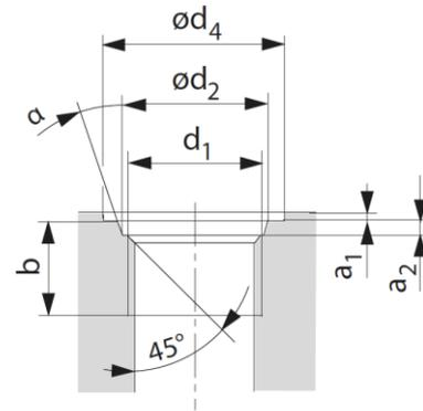
Figure 19: UNF, metric thread
