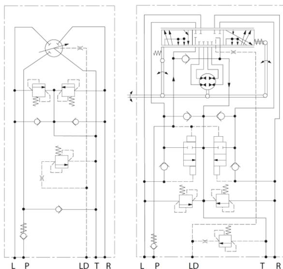
**Figure 5: LAGU LDA / NR schematic**
