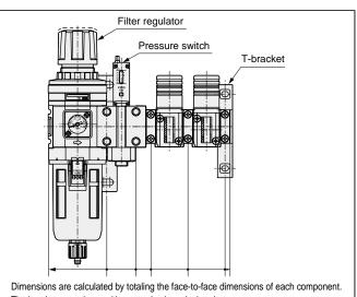
The bracket mounting position can also be calculated.
