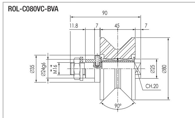
Radial load: 1000 N max. - lifetime lubrication **Fig. 91**
