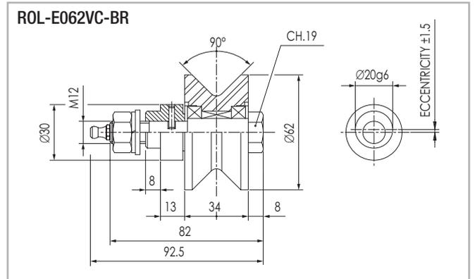
Max. Load: radial 700 N/axial 280 N - Optional lifetime lubrication
