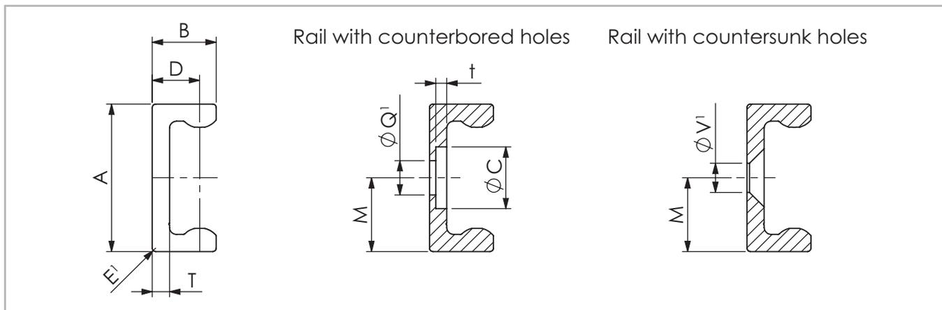
Q' Fixing holes for Torx® screws with low head (custom design) included in scope of supply
