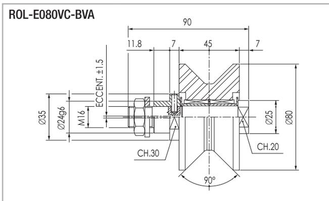
Radial load: 1000 N max. - lifetime lubrication **Fig. 92**
