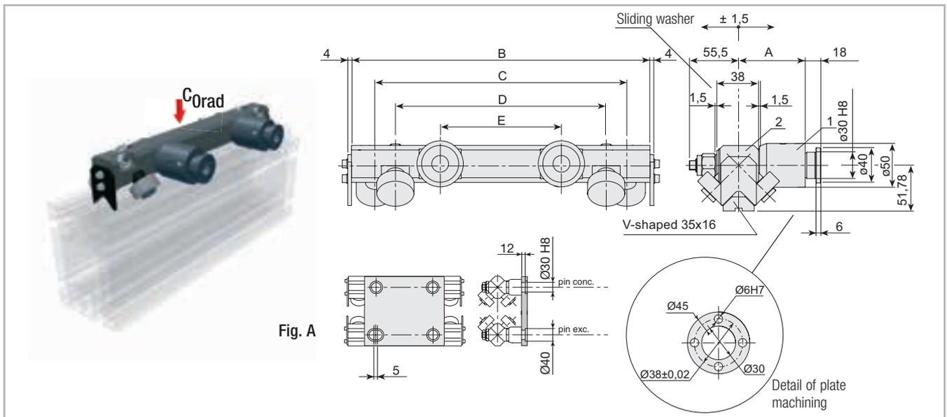
Important: remove the space washers to enable self-alignment of the roller slide sliding washers
