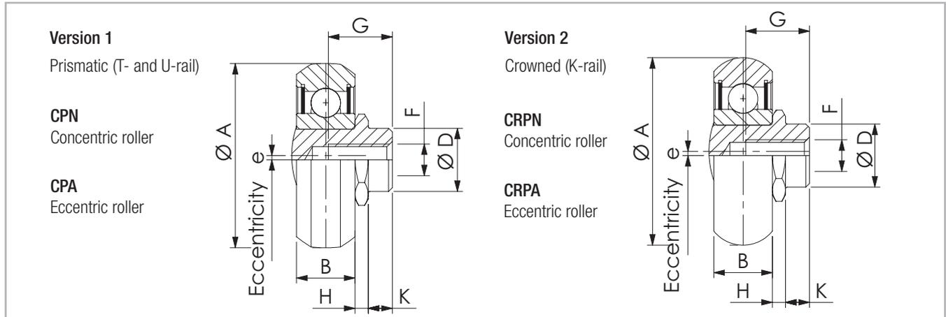
Seals: 2RS is the splash-proof seal, 2Z (2ZR for size 63) is the steel cover disc
