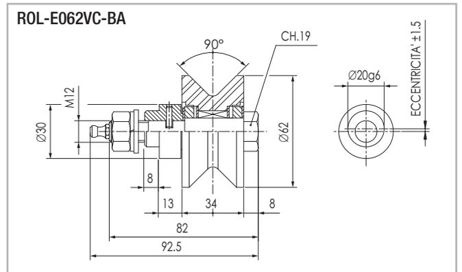
Max. radial load: 700 N - Optional lifetime lubrication
