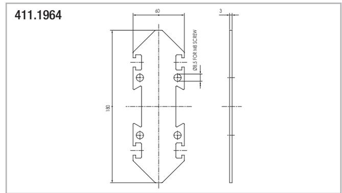
Fishplate for mod.2 Rack mounting on SR180, SR250 T grooves
