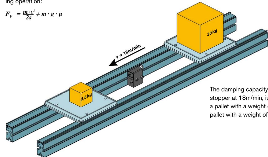
The damping capacity, e.g. of a DBS-90 stopper at 18m/min, is sufficient for both a pallet with a weight of 5 kg and for a pallet with a weight of 50 kg.
