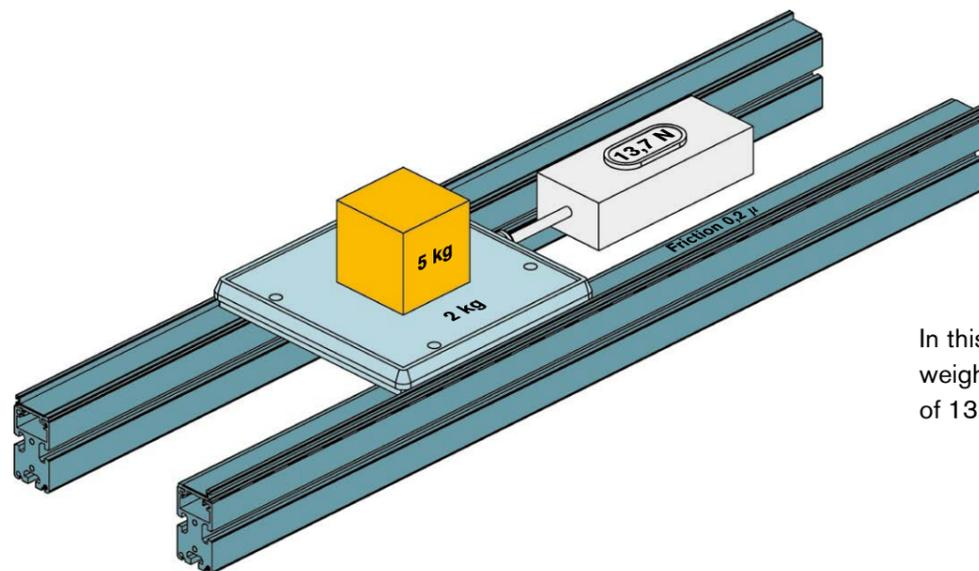
In this example, a pallet of total weight 7 kg exerts a propelling force of 13.7 N on a double belt conveyor.
