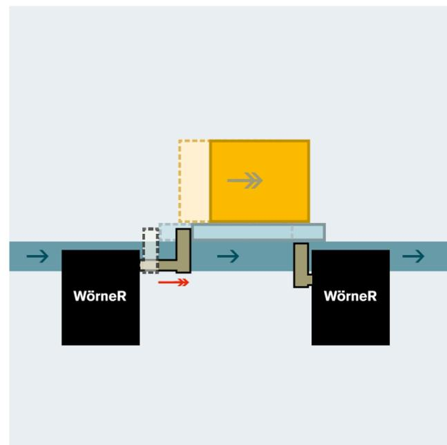
Displacement stops are integrated at a transverse section that connects more than two longitudinal sections. They take over transport control at line crossings and stop pallets e.g. on lifting transverse units. Thus the pallets can be transferred from a transverse to a longitudinal section. The displacement stop can perform different functions:
