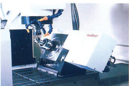
Manually swivelling NC dividing head with controlled rotating axis and hydraulic clamping
