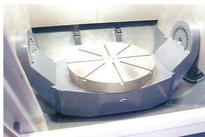
2-axis NC rotary table with torque drive in the rotating and swivelling axes
