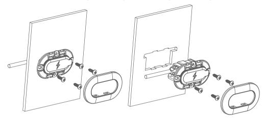
2. Embedded Installation: Using 2 Upper/Lower mounting points for square mounting plate
