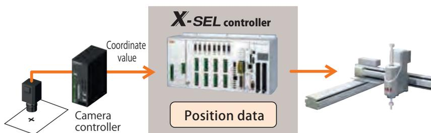
(3) While communicating with a vision system via Ethernet, communication with another network is possible.
