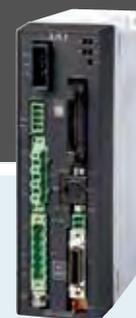
Position Controller for Single-axis Robot/Cartesian Robot/RoboCylinder
