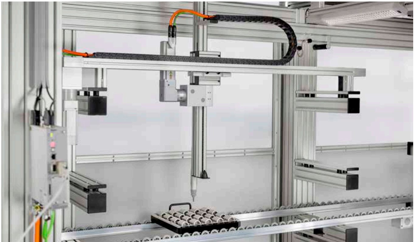
Fig.: Linear Unit KRF 8 80x40 ZR, drive side on left (0.0.641.21) with Drive Set KRF 8 ZR AP/WP 60 (0.0.673.31), Gearbox AP 60-5 (0.0.666.12), Motor SE 60-150-3-60-R (0.0.666.02), Linear Unit LRE 8 D10 80x40 ZS K light (0.0.679.91) with Drive Set Rack 8 AP/WP 60 (0.0.673.33), Gearbox WP 60-3 (0.0.666.14), Motor SE 60-150-3-60-R-B (0.0.665.99), Controller C 1-05 (0.0.668.63)
