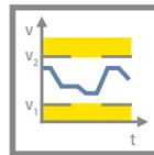
Monitors that the drive observes a defined speed limit. In the event of an error, SS1 is triggered.
