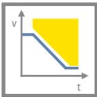
The drive is brought to a standstill by controlled braking and subsequently remains in controlled standstill. The control functions of the drive are maintained.
