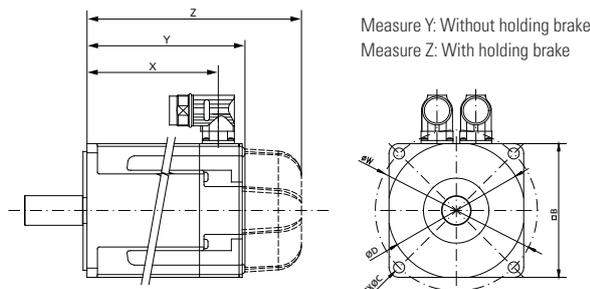
All measurement specifications in mm Measure Y: Measurement without holding brake, Measure Z: Measurement with holding brake
