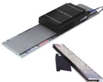
Directly coupling a linear motor to the driven load offers many advantages, including eliminating all mechanical transmissions, such as ball/lead screws, rack & pinions, belts/pulleys, and eliminating gearboxes. This in turn also eliminates backlash and compliance, and other problems associated with these mechanical transmissions.
