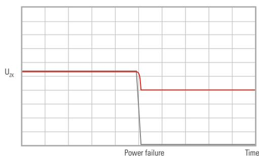
Voltage on the DC-Link During Power Failure
