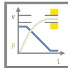
Monitors the stop position reached and triggers SS1 in the event of deviations beyond the specified limits. The control functions of the drive remain active.
