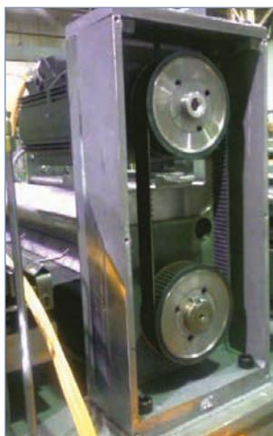
Press feed machine built with a conventional servo motor, gearbox, belt and pulleys.
