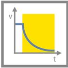
STO safely interrupts the power supply to the motor in the servo drive. The motor becomes torque-free.
