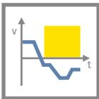
The SDI function ensures that the drive can only move in a defined direction. In the event of an error, SS1 is triggered.
