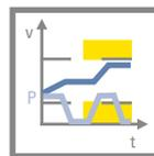
Monitors the relative position of the drive with respect to the current position when activating the SLI function. SS1 is triggered when the prescribed limit value is reached.
