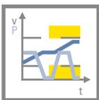
Monitors the absolute position of the drive. If the limit value is reached or the brake torque is too low to keep the drive within the limit value, SS1 is triggered.
