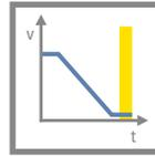
The drive is brought to a standstill by controlled braking. Then the power supply to the motor is safely interrupted and the motor becomes torque-free.
