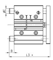
Dimensions L3 and B change according to the different strokes of QCB. For out of standard intermediate strokes (ex. stroke 35), consider the immediately higher stroke dimensions (ex. stroke 40).
