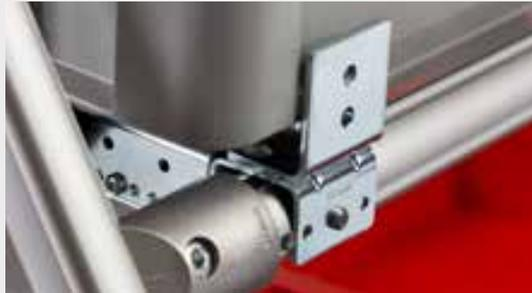
As Roller Conveyor St Stop H43 is not mounted to a cross-member, users can build roller conveyors that project outside a frame and thus reduce reaching distances. Light transport boxes are brought safely to a halt. The stop must be screwed to the Roller Conveyor St D30.
