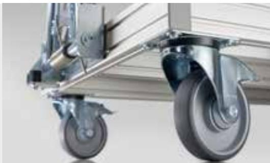
Swivel and Fixed Castors can be fixed to frames made using Line 8 profiles via the four holes in the integrated connecting plate. Alternatively, the Castors can be fixed to two parallel Profiles 8 D30. These tubes from Profile Tube System D30 feature an integral Line 8 groove. The corresponding Fastening Set 8 for Castor swivel/fixed makes installation easy.
