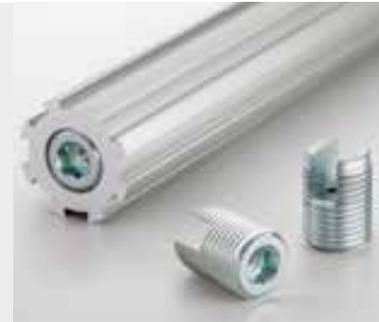
Prior to installation, screw a suitable Hexagon Socket Head Cap Screw with lock nut into Threaded Insert, Profile Tube D30 heavy duty. Use the screw and lock nut to drive the Threaded Insert into the end face of the Profile Tube D30 heavy duty. The Threaded Insert is self-tapping. Next, loosen the lock nut and remove the screw to free up the thread.
