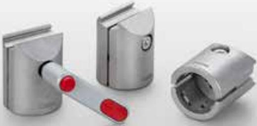
The universal and secure 90° connection: Fastener D30 made of die-cast aluminium creates a mechanically locked connection with the contour of a Profile Tube D30 or Profile 6 D30.
