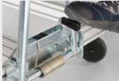
Drawbar Locking Lever 38 keeps coupling elements neat and safe. It holds the Drawbar securely in a vertical position, which is particularly advisable when using the version without a self-lifting mechanism. The foot-operated lever ensures the locking lever can be released without having to stoop down.
