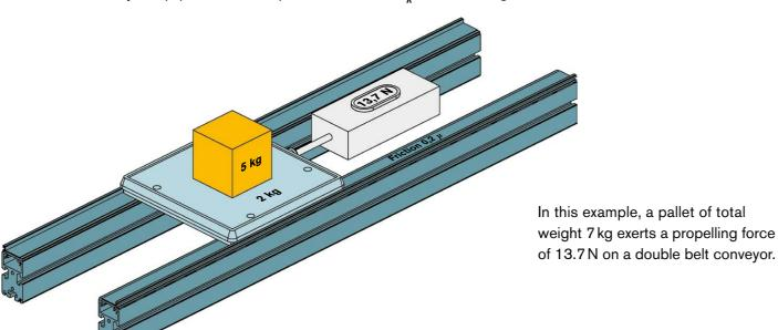
The product brochure and data sheets indicate the maximum propelling force against which the stopper can reliably lower during long-term operation. The propelling force in your system must be less than the specified value.
