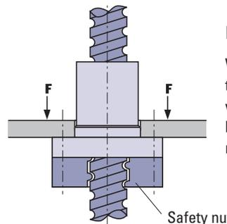
Installing a safety nut
