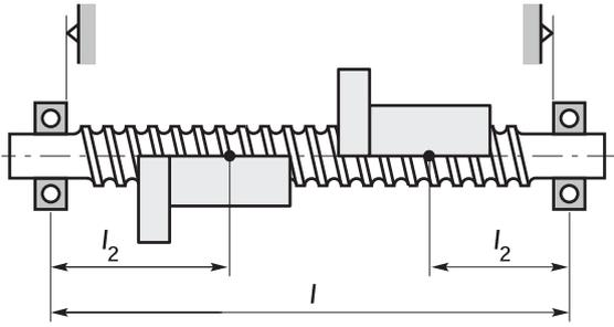
$R_{s2} = \frac{A \cdot E}{l_2 \cdot 10^3} \cdot \frac{l}{l - l_2} \quad [N/\mu m] \rightarrow l_2 \leq l/2$ <p><math>R_{s2, min} \text{ at } l_2 = l/2</math></p> |
