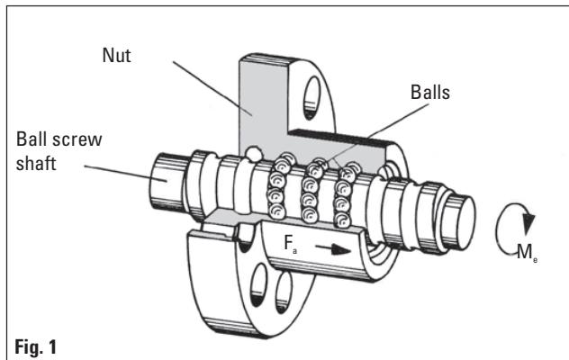
Action: Torque  $M_a$  → Reaction: Force  $F_a$
