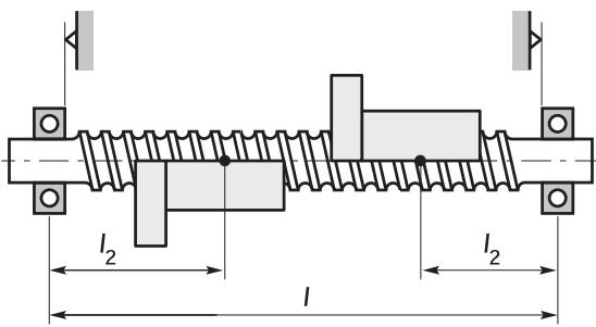
$$R_{s2} = \frac{A \cdot E}{l_2 \cdot 10^3} \cdot \frac{l}{l - l_2} \quad [\text{N}/\mu\text{m}] \rightarrow l_2 \leq l$$
