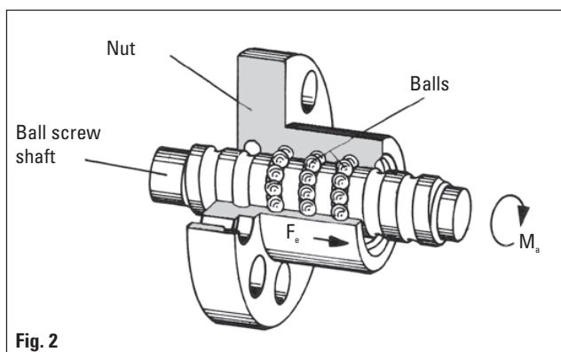
Action: Force  $F_a$  → Reaction: Torque  $M_a$
