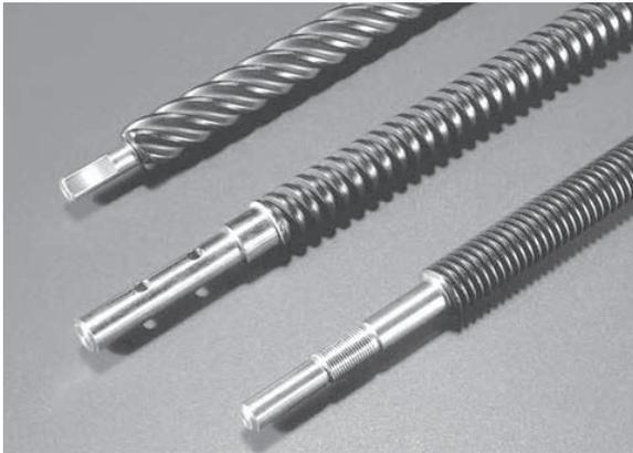
A PTFE coating comprises a dry coating, forming a lubricating and barrier layer between the metal substrate and the polymer nut or ball nut. This means that the application of an additional lubricant that must be renewed is unnecessary in many cases.
