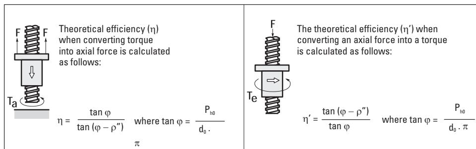
The theoretical level of efficiency is reduced by around 5% to make allowances for operating influences such as speed, temperature and lubrication. If the ratio of load  $F$  to dynamic rated load  $C_{am}$  is less than 0.5, a further reduction is made based on the load factor  $f_f$  (see table below).
