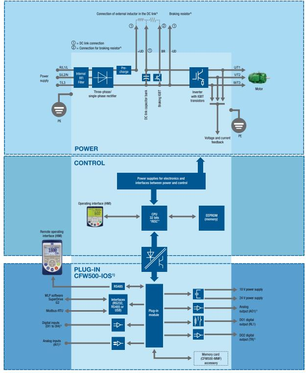
Notes: 1) The number of inputs and outputs (analog and digital), as well as other resources, may vary according to the plug-in module used. For further information, refer to the CFW500 user manual. 2) Not available for size A.
