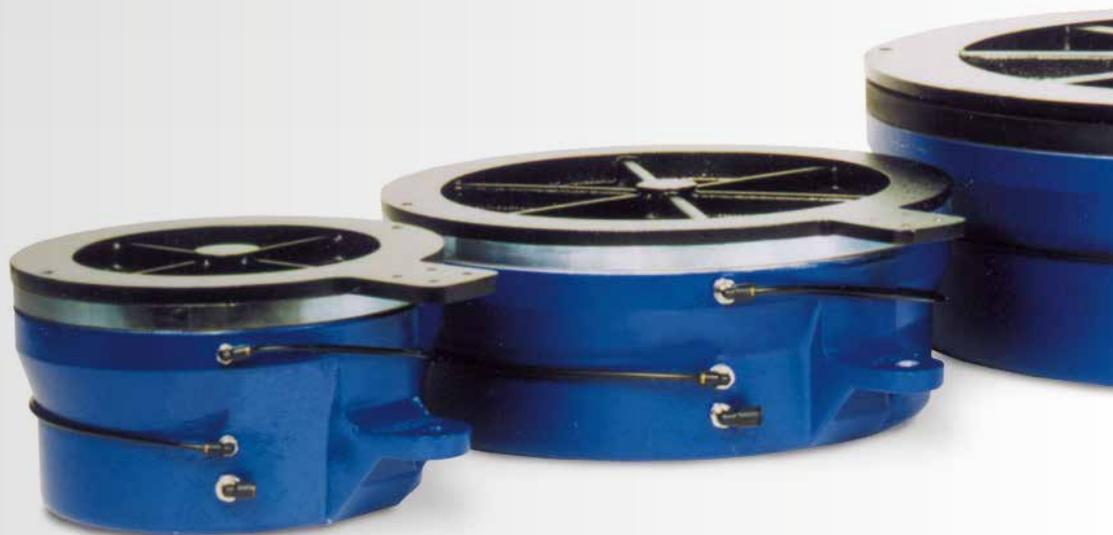
Standard PAL isolators have a natural frequency of up to 1.7 Hz – depending on the height of the isolator. Even lower natural frequencies (up to 0.5 Hz) are possible for isolators manufactured according to customer specifications.
