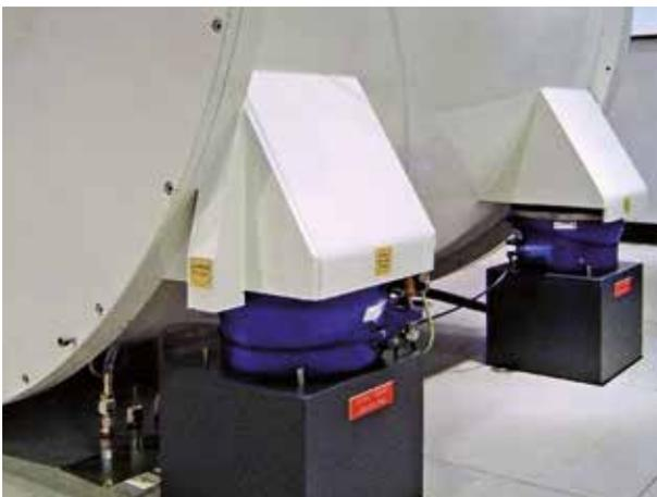
A measuring machine as an example of receiver isolation
