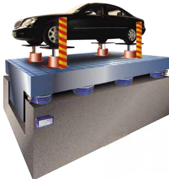
Test benches, example: street simulation test bench
