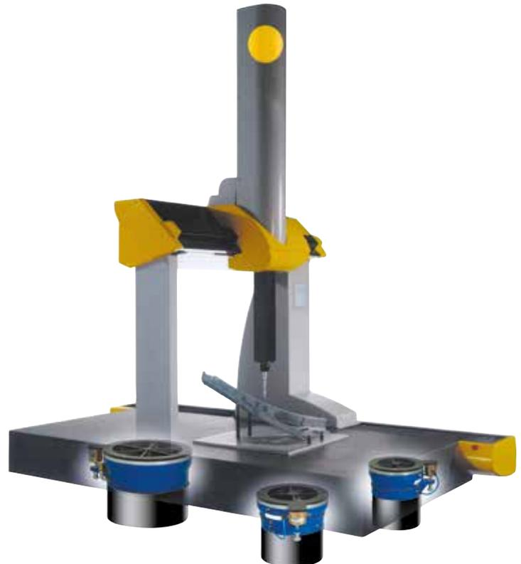
Measuring tables, example: coordinate measuring machine
