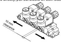
(4) Raise the pressure gauge side and pull the block toward the pressure adjustment knob to remove it from the DIN rail. When the DIN rail brackets on both sides are slid 2 mm or more from the end block, the entire manifold block can be removed.
