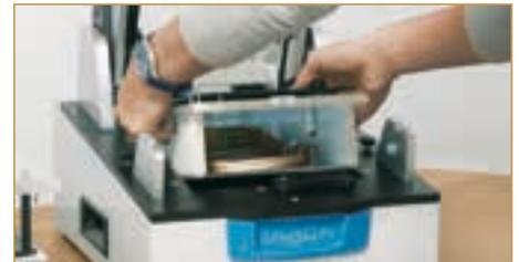
2.) Unlock the Probe Plate Unit at the front by means of the hand lever, lift upwards and take it out of the mounting
