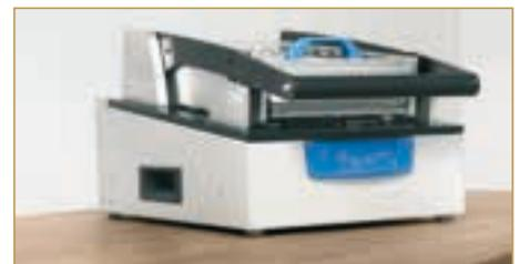
5.) Slide Probe Plate Unit into the mounting, lock at the front by means of the hand lever and close Pressure Frame Unit
