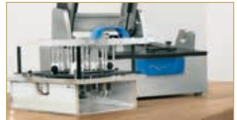
3.) Move Safety-pusher to the left, press locking bar and take out Pressure Frame Plate from above
