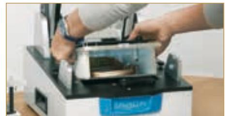
4.) Move Safety-pusher to the left, press locking bar and put in Pressure Frame Plate latching from above
