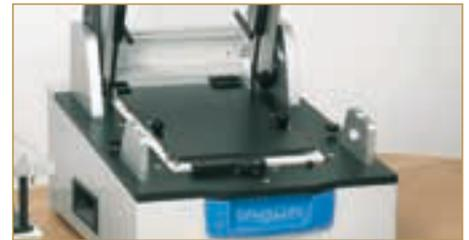
1.) Lift up the handle upwards and open Pressure Frame Unit completely
