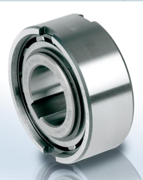
Type ASNU is a roller type freewheel non-bearing supported. Bearings are required to support axial and radial loads. Lubrication and sealing must also be provided by the installation. Nominal outer diameter is the same as a series 63.. ball bearing.
