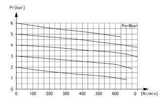
Flow diagram for models: M004-R00 Pa = Inlet pressure (bar)
