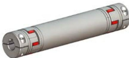
*Easy radial mounting with 2-part coupling hubs, replacement of toothed spiders without displacement of the drive shafts. Lengths up to 4 meters are possible without pillow block bearing are possible depending on revolution speed and size. Low mass moment of inertia due to aluminum material. Combination with other hub versions are possible. Bore size to ISO-fit H7, key to DIN 6885 Bl. 1 – JS9.*
