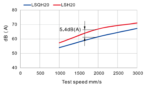
Pic.2 - Noise degree comparison test between LSQH series and LSH series.
