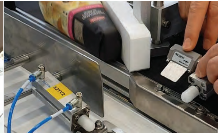
Air knife for defective parts' discard
