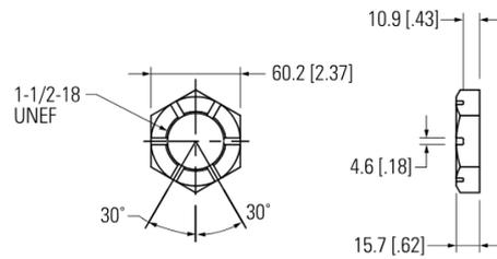
Figure 26 Slotted hexagon nut
