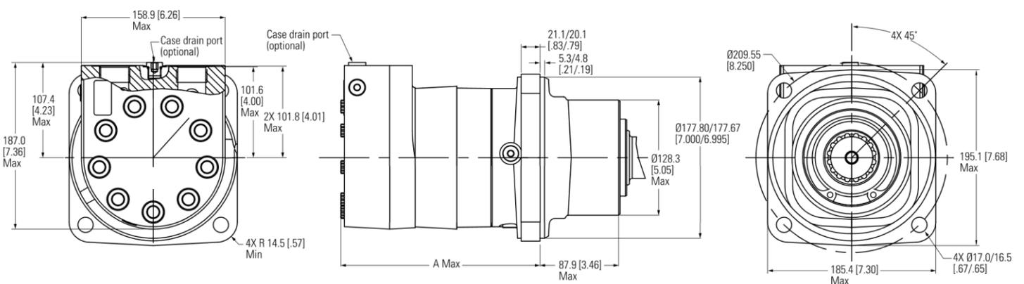
Figure 16 Wheel Mount Open loop
