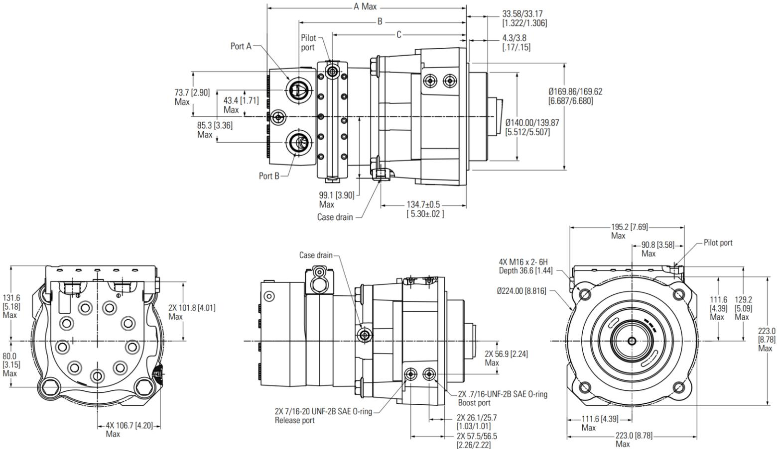
Figure 48 Brake motor two speed closed loop
