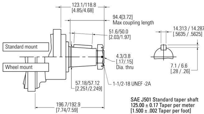
Figure 24 2 1/4 inch tapered shaft
