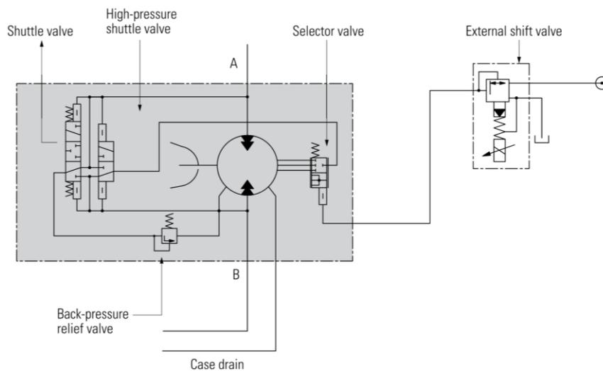
Figure 44 Two-speed circuit
