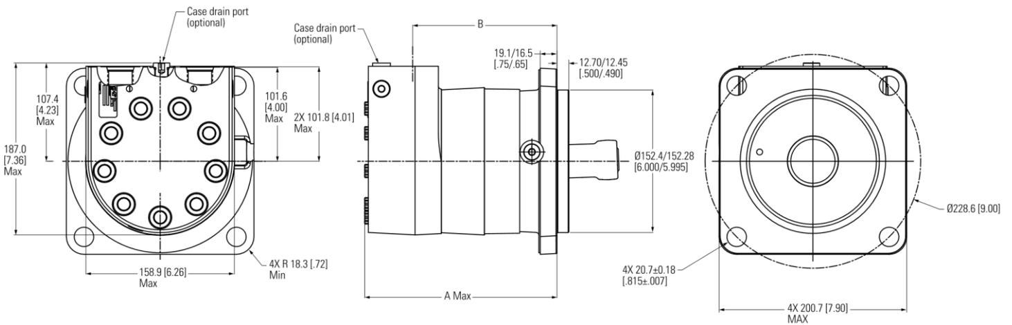
Figure 20 Bearingless mount open loop
