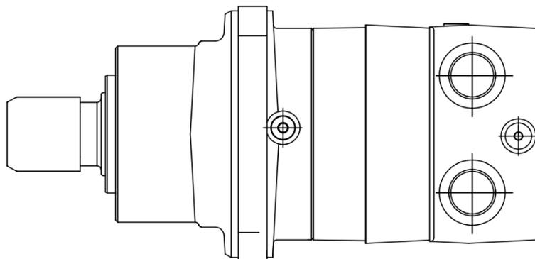
Figure 2 Wheel motor
