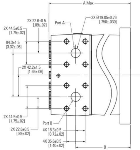
Figure 14 Wheel Mount manifold interface
