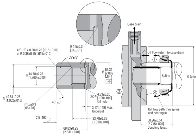
Figure 21 Install instruction bearingless mount
