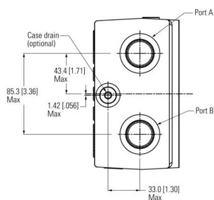
Figure 18 Bearingless mount open loop configuration
