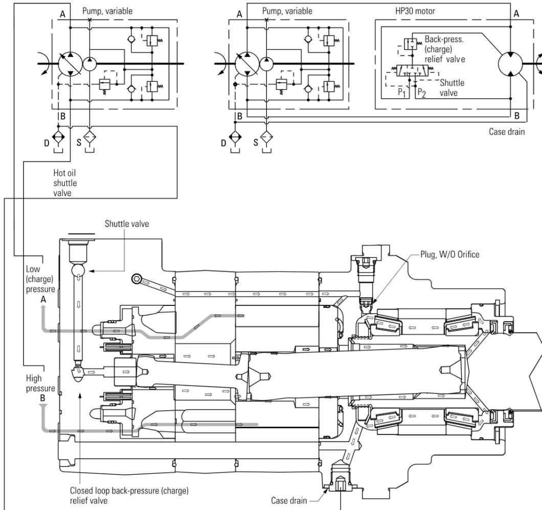
Figure 41 Closed loop circuit
