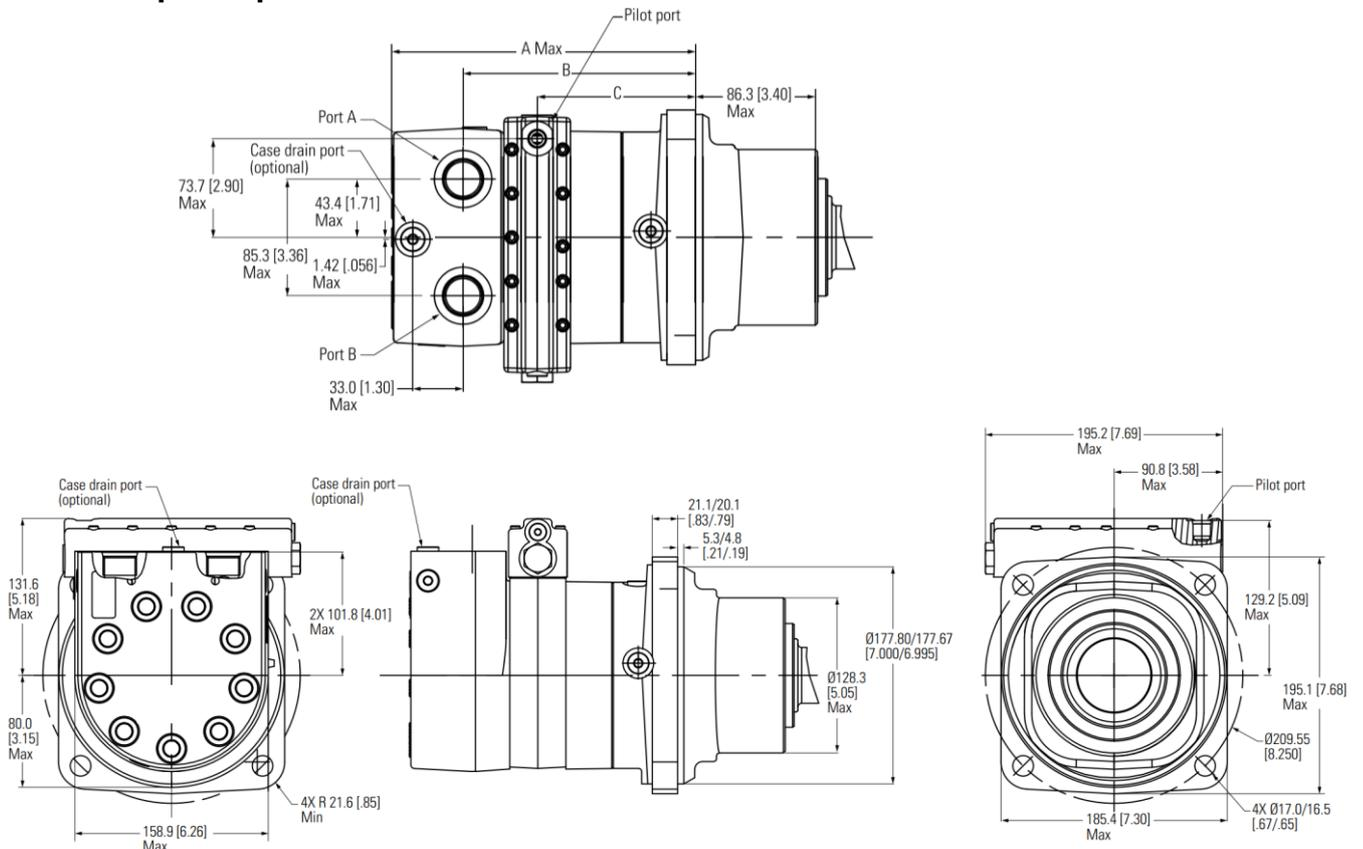
Figure 37 Two speed motor wheel mount open loop
