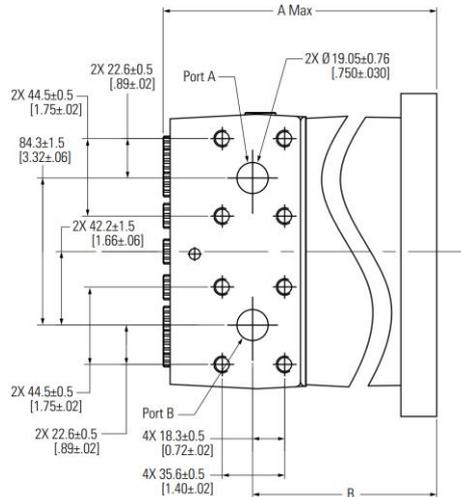
Figure 11 Standard mount Manifold Interface
