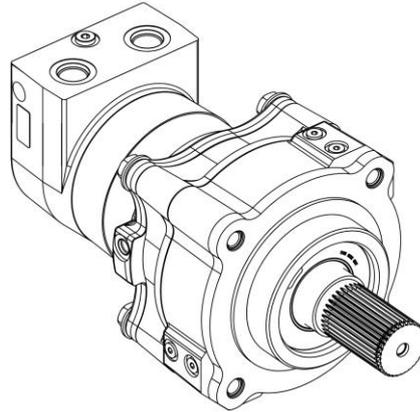
Figure 46 Brake motor
