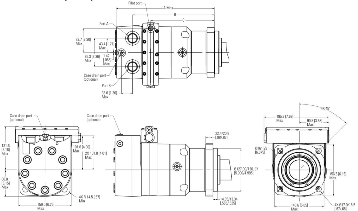
Figure 34 Two speed standard open loop
