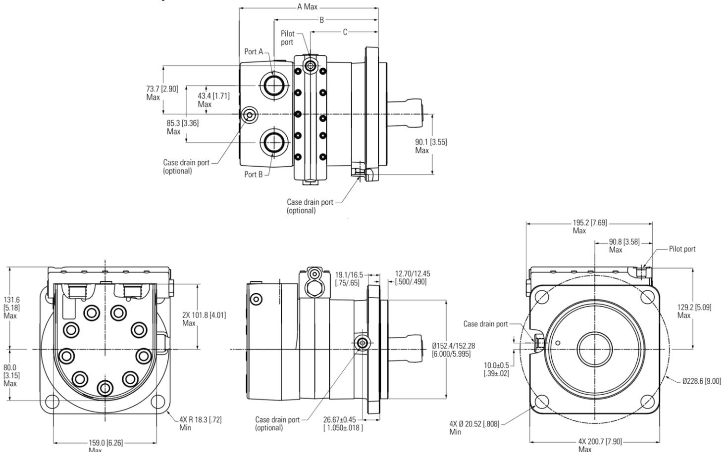
Figure 38 Two speed bearingless closed loop
