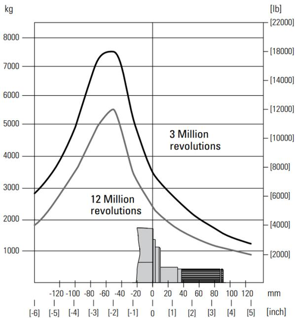
Figure 49 HP 30 Brake curve
