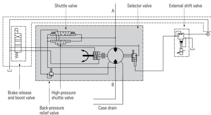
Figure 45 Two speed brake motor circuit
