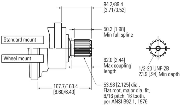
Figure 22 2 1/8 inch 16 tooth splined shaft
