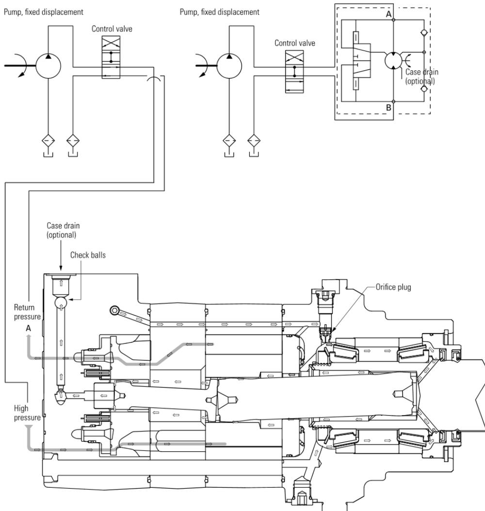
Figure 43 Open loop circuit
