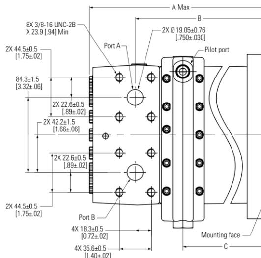
Figure 31 Two-speed standard motor manifold interface
