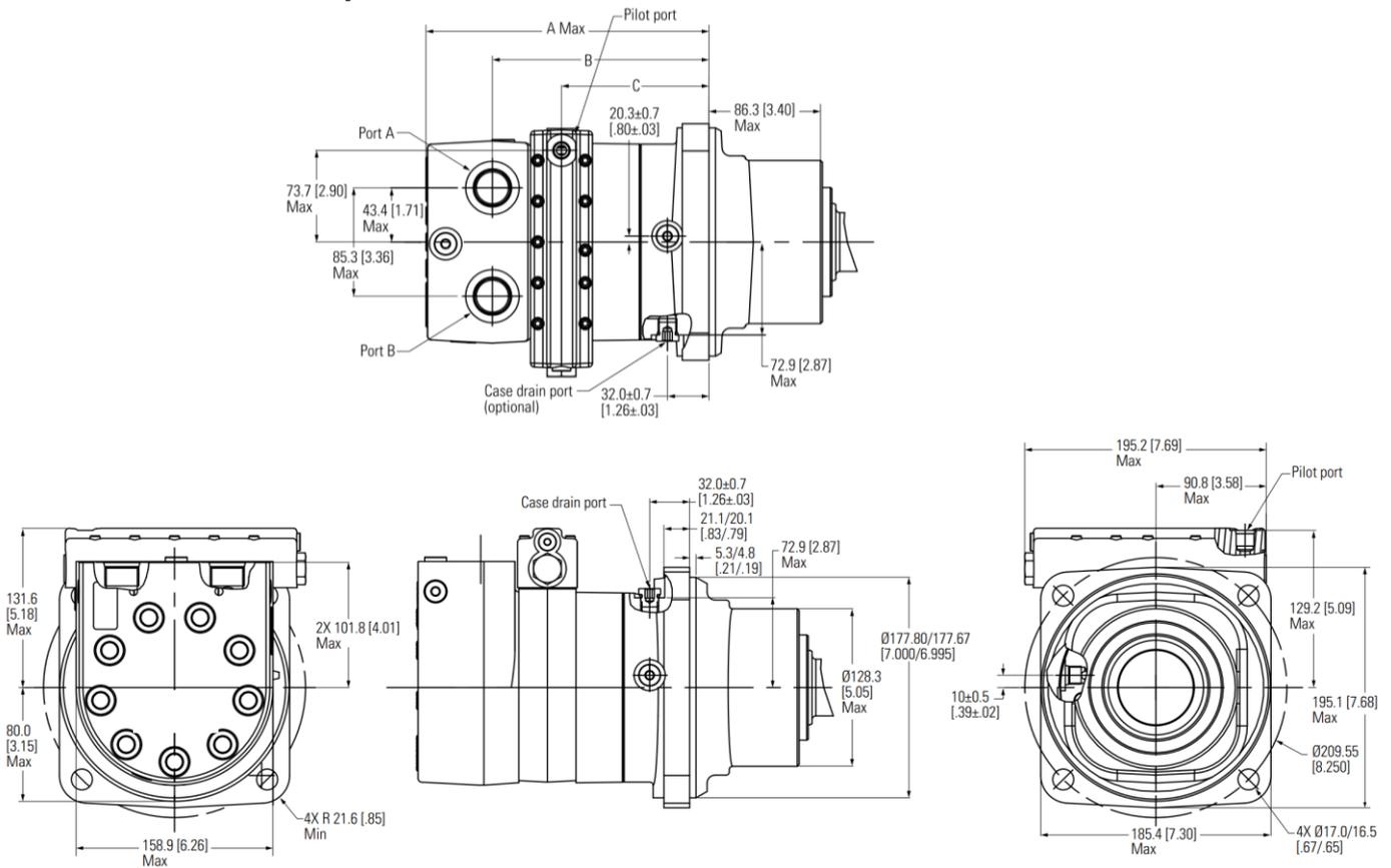
Figure 36 Two speed motor wheel mount closed loop
