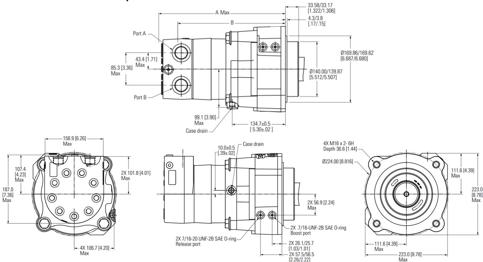
Figure 47 Brake motor single speed closed loop
