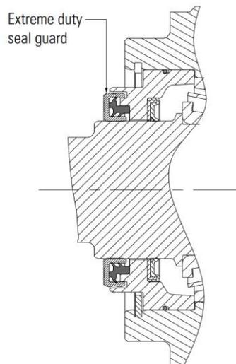
Figure 4 Extreme duty seal guard
