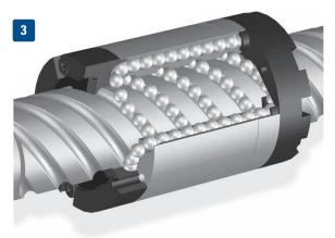
**End-Cap Return** The balls are recirculated via two special end caps and return channels integrated into the nut.
