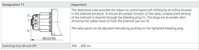
The switching times shown are valid for viscosity  $\nu=32$  mm²/s (156 SUS) and nominal voltage. They depend on working pressure and flow rate of the directional control valve.
