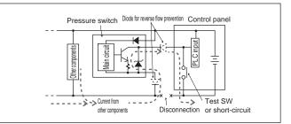
Take the following measures to prevent damage caused by reverse current:
